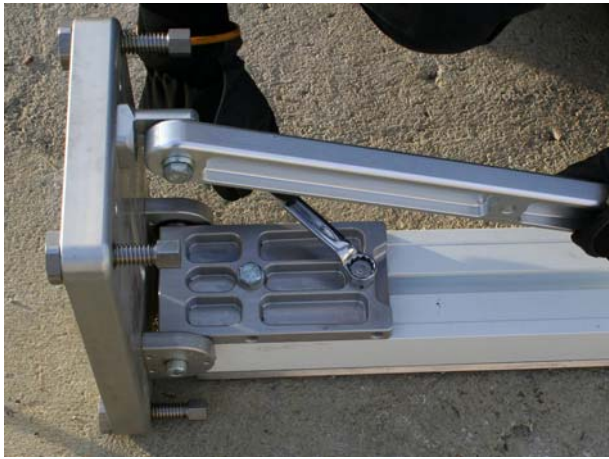
c. Tighten the two bolts on the lower clamp.
